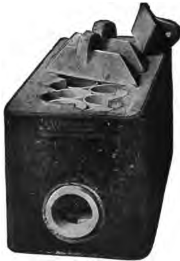
FIG. 16.—GASOLENE-BURNING CRUCIBLE FURNACE.
